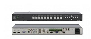
The VP-436 is a 7-input scaler/switcher for composite video, s-Video (Y/C), component video, computer graphics video and HDMI with unbalanced stereo and S/PDIF audio signals. It scales the selected video signal to a computer graphics or HDTV output resolution, embeds the audio and outputs an HDMI signal.
